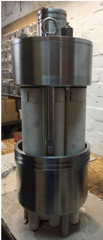
Assembled Replacement Hydrocyclone Cartridge
